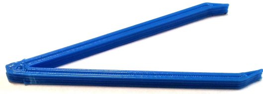
Figure B.12: Tweezers to test flexible designs (frequently used to remove excess extrusion produced during self-cleaning)
