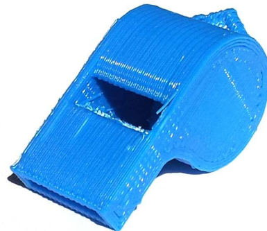
Figure B.11: Whistle (with pea printed inside) to test precise, air-tight objects with simultaneously printed sub-components
