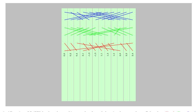
Figure 8: Allocation of SpiNNaker boards to cabinets and racks and the wires between them. Colour key: North, East, South West
